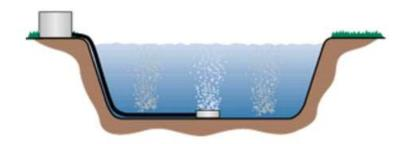
Aerators pump air down the bottom of a pond & the air bubbles up through the water. Most people don't even notice the bubbles "boiling" up over the aerator head.
